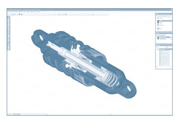
Manipulate 3D data to create a cutaway that depicts either a precise part or several components.
